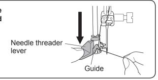
Fully turn the needle threader lever to the rear, and pull the thread through the needle threader slot.
