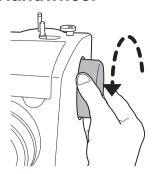
• Use the handwheel to manually raise and lower the needle.
