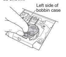
Insert the right side of the bobbin case into the hook so that part © on the bobbin case is to the left of part d on the sewing machine.
