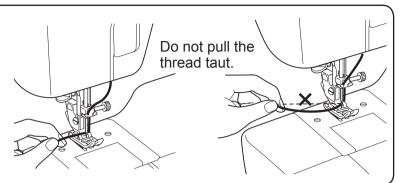
2 Lightly pull the upper thread with your left hand to pull up the lower thread.
