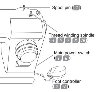
5 Slide the thread winding spindle in the direction of the arrow until it snaps into place.
