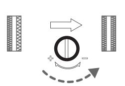
If the stitches are loose on the left side of the buttonhole, turn slightly in the "+" direction.
