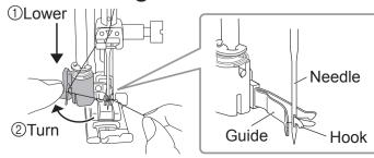
The hook is within the guide. The hook passes through the needle, catches the thread, then pulls the thread through the needle.
