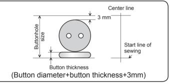
Align the buttonhole foot division line closest to you with the guide line, and lower the presser foot to the start line of sewing on the fabric.
