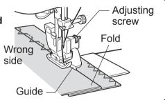
After sewing, pull out the tacking, and fold out the fabric.
