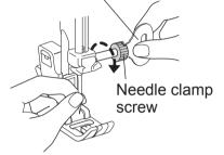
Face the flat surface of the needle to the rear and insert until it makes contact with the pin.
