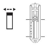
Raise the needle to the highest position, set the pattern dial to "3", sew the right side and stop at the line marked on the fabric.
