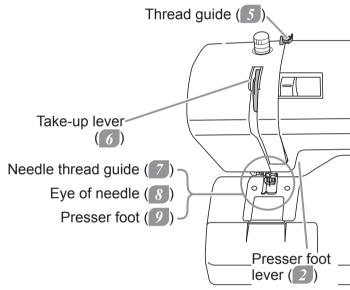
From the front. pass the thread through the eye of the needle.
