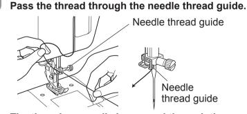
The thread can easily be passed through the needle thread guide by holding the thread in your left hand, then feeding the thread with your right hand, as shown.
