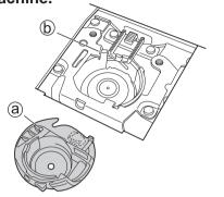
With the bobbin case tilted to the left, insert the left side of the bobbin case into the hook, as shown.
