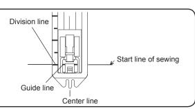
Raise the needle to the highest position, set the pattern dial to "1", sew the left side and stop at the line marked on the fabric.
