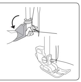
Pull the thread loop that formed behind the needle, and then pull about 15 cm of thread to the rear.
