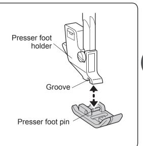
2 Lower the presser foot lever to secure the presser foot.
