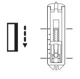
Raise the needle to the highest position, set the pattern dial to "4", and sew 5 to 6 bar-tack stitches.
