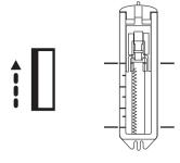
Raise the needle to the highest position, set the pattern dial to "2", and sew 5 to 6 bar-tack stitches.
