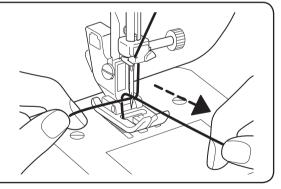
Align both threads, pass them through the groove (arrow) and under the presser foot, and then pull out about 15 cm of thread to the rear.
